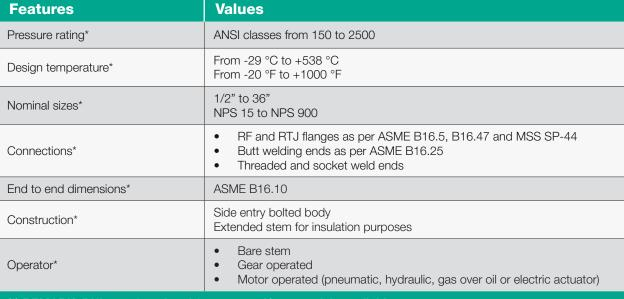
(\*) REMARK: Different functional features and/or materials available on request. Stated temperature ranges are the maximum for which the standard equipment's full performance is fulfilled. (\*\*) REMARK: If necessary, proper material pups can be welded to the valve to fit connecting pipe material.
